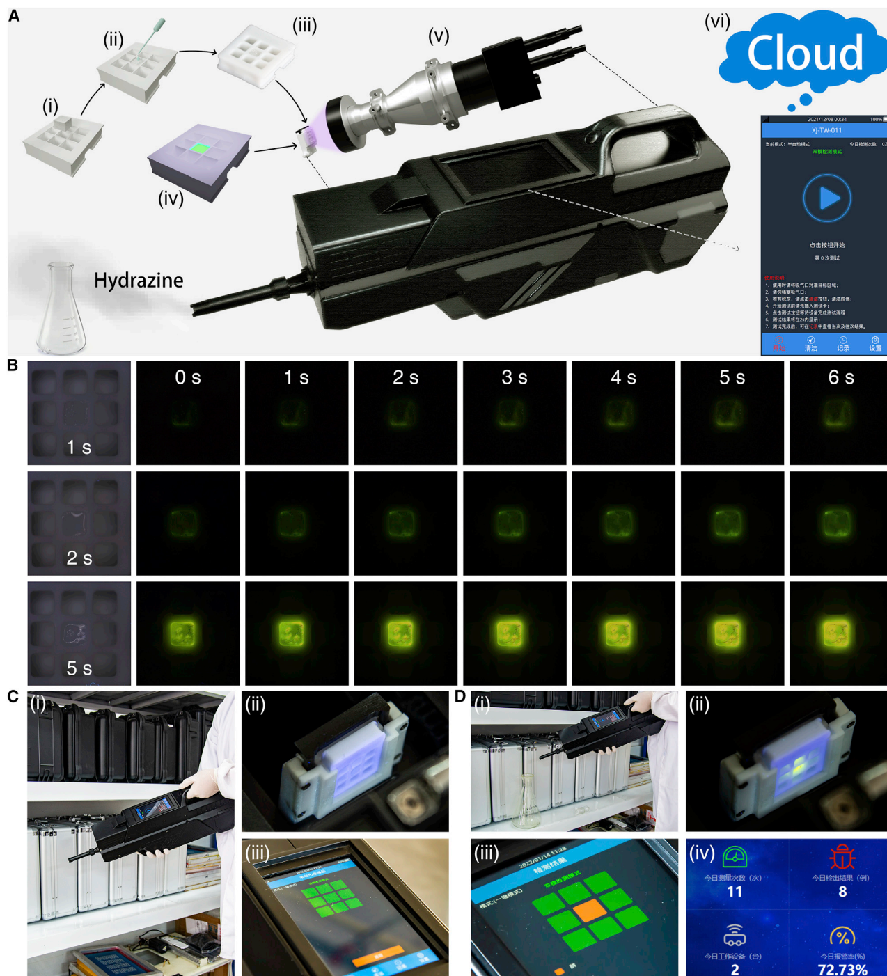
Figure 5. The F-CN probe-embedding portable detector for the fast and on-site detection of hydrazine vapor
